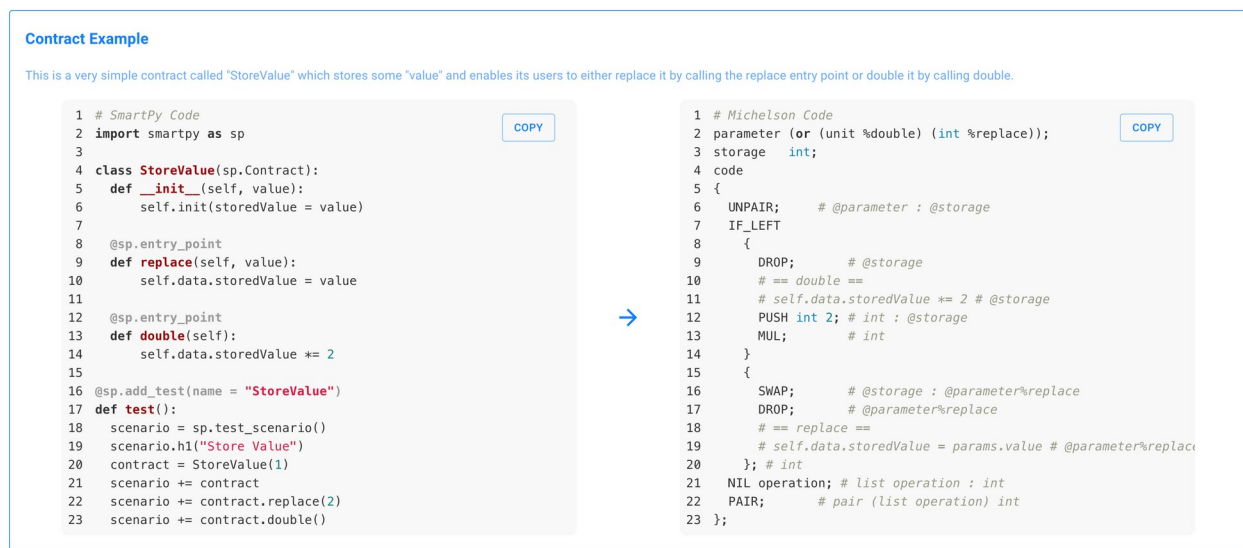
Figure 1: A comparison of a simple smart contract in Python (left) and Michelson (right) 13
